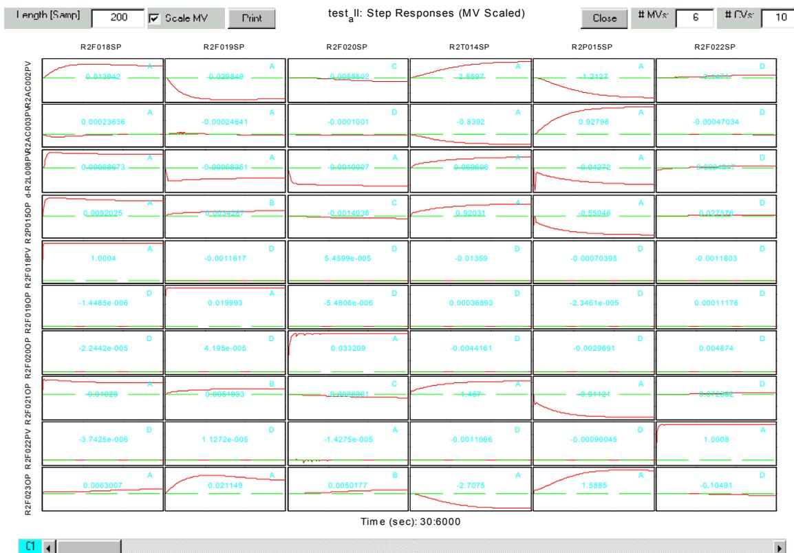
Figure 4.5 Model step responses, open loop identification,
