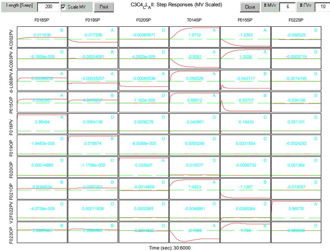
Figure 4.7 Model step responses, closed-loop identification
