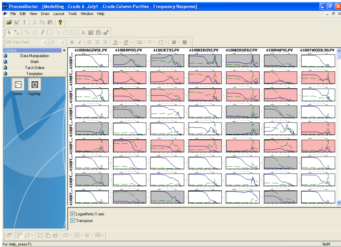
Figure 4.5 Frequency response plots for selected models. (pink background: Model expected but model quality not satisfactory, white background: model expected and good quality model identified, grey background: no model expected)
